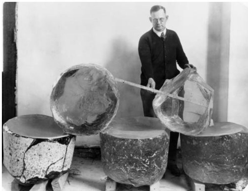
Figure 4. These large masses of optical glass were manufactured at the Bureau in 1919.
